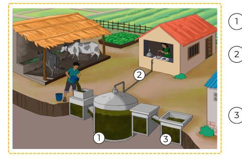
The mixture is fermented in a tank.
