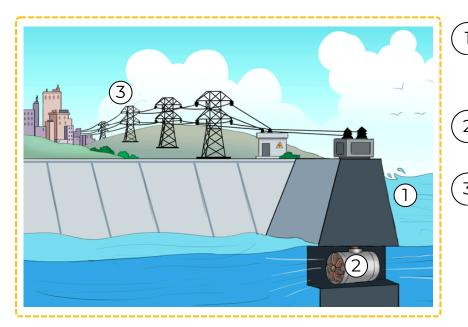
The water that comes in during high tide is used to turn turbines.
