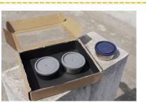
Place the black and one unpainted container inside the solar cooker. Place another unpainted container outside the solar cooker in sunlight. This will be the 'control'.
